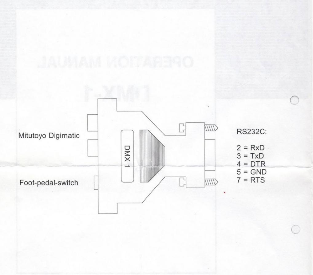
The interface DMX-1 is been used to connect 1 measuring instrument with a DIGIMATIC data - interface to the the serial interface of a standard PC.
