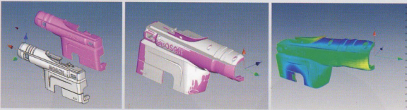
Fig. 6 CAD model (left) with CT data and evaluation of geometry deviations with default toleration field (middle and right).
