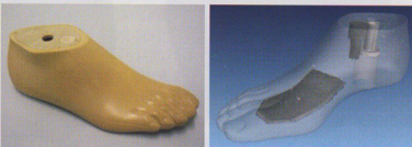
Fig. 8 Epithetic foot and obtained 3D model (visible transparency of lower density material – soft surface plastic and wood).
