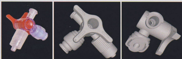
Fig. 3 CAD models of the multidirectional valve – presentation of the reverse engineering.
