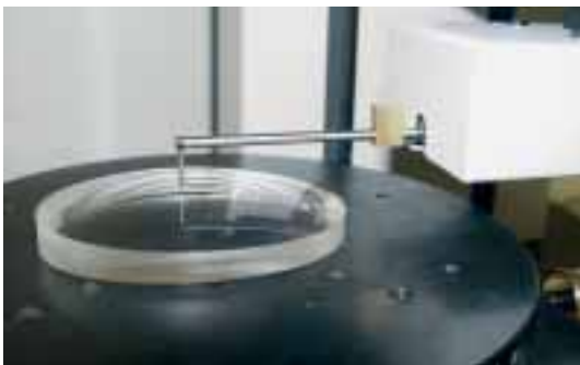
Example application: asphere measurement on a lens
